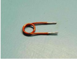
[ ] Position and solder T1 primary and secondary windings elevated from the surface of the board as shown. The spacing between the coils should be approx. 1/8" (3mm) This will allow for spreading or adjustment between the two, during the setup procedure. For Aircraft band use holes marked 1 and 2 for the primary.
