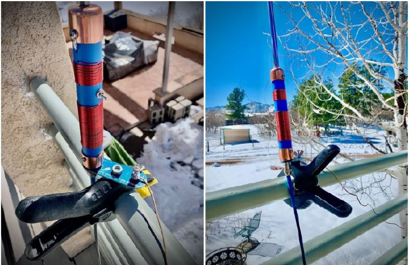
Steve Galchutt (WG0AT) mounting his with a Harbour Freight clamp for railing, tree branch, or picnic table.
