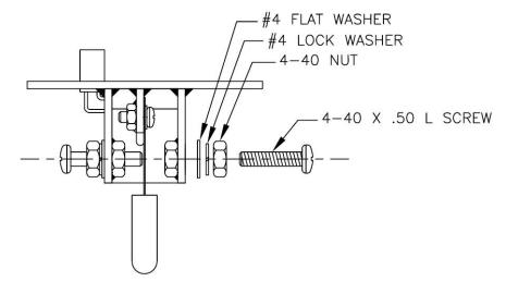
This completes the paddle assembly. Use the two 4-40 thumbscrews to secure the paddle to the transceiver.
