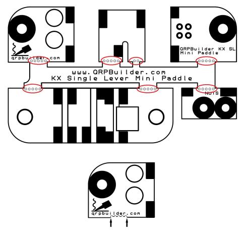
None of these 7 break areas should protrude beyond the edge of any of the boards. If they do, lightly rub on a piece of emery paper if needed. A light touch is all that is required. Like shown below.
