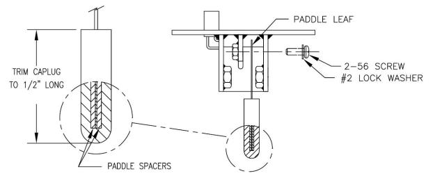
Cut the vinyl caplug lever cover 1/2" long from the closed end. Scissors will work easily. Cut the piece of 1/2" wide plastic into two 7/16"" long pieces. Sandwich the paddle lever between the plastic spacers and slide the caplug over the end of the paddle leaf.
