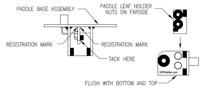
Next, the two **brass** 4-40 nuts need to be permanently soldered to the "inside" of both the contact holders. Use the 4-40 x 3/8"L SS screw, and, a #4 lock washer to hold them in place, and solder the brass nuts to the PCB. *The lock washer insures that the nut will be flush with the PCB when it is heated.* Rub the face of the nut on some scotchbrite or emery paper to clean up the surface contacting the PCB.
