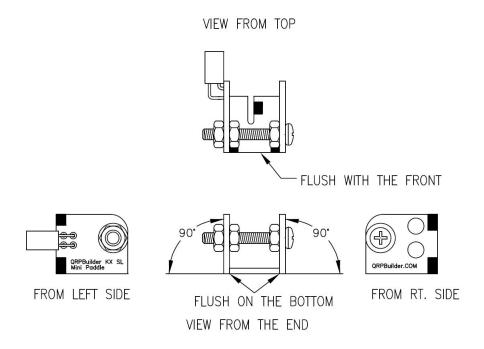
Once all this is aligned and secured, place on a flat surface, and put a "small" tack between each contact holder and the support. *Leave the support screw in place.*
