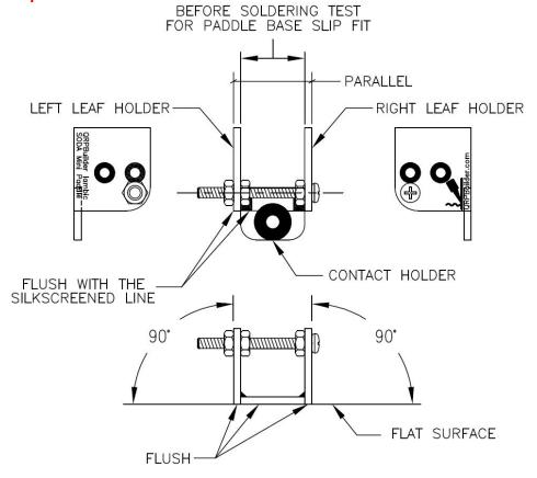
Mate the previous assembly to the Paddle Base as shown in the figure below. The Paddle Base should be a slip fit between the two leaf holders. Tack one small joint and check for alignment. When you are satisfied with the alignment, lightly tack all the other points. Finish soldering all the pads, including the joints between the leaf holders and the Contact Holder. You may now remove the 4-40 screw and nuts.
