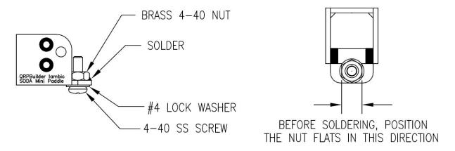
Solder the brass nut to the inside of the Paddle Base as shown below. Then remove the screw and L.W.
