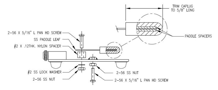
[ ] Mount each Paddle Leaf, spaced off the pcb, with two .12" thick nylon spacers. Use the hardware In the order as shown in the graphic.
