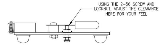
[ ] Cut the vinyl caplug lever cover 5/8" long from the closed end with scissors or a razor knife. Cut the 1/2" wide plastic into four 9/16" long pieces. Sandwich the paddle lever between the plastic spacers and slide the caplug over the end of the paddle leaf.
