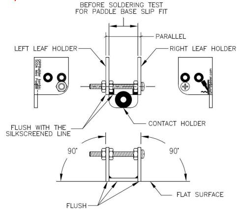
Mate the previous assembly to the Paddle Base as shown in the figure below. The Paddle Base should be a slip fit between the two leaf holders. Tack one small joint and check for alignment. When you are satisfied with the alignment, lightly tack all the other points. Finish soldering all the pads, including the joints between the leaf holders and the Contact Holder. You may now remove the 4-40 screw and nuts.
