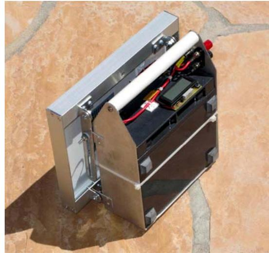
In the left picture you see a small board attached to the side of the battery. That is a 12v - 24v buck booster used to power my small magnetic loop antenna tuning motor.
