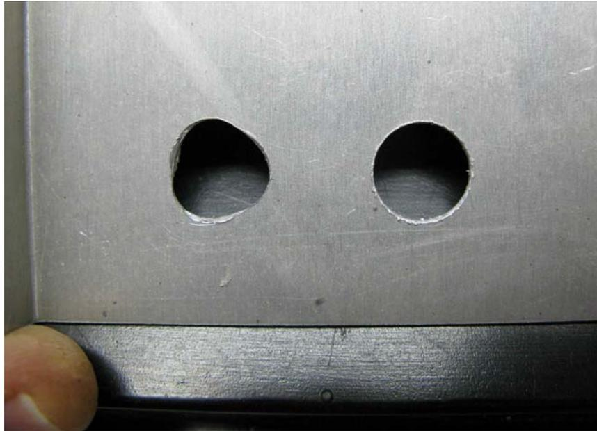
Compare the two holes above, in a piece of .050" thk. aluminum. Both holes were drilled with a 1/2" dia. drill at about 150 rpm, with a wood support on the backside. The hole on the left was drilled with a standard twist drill, the one on the right with a modified tip. Neither hole has been de-burred.
