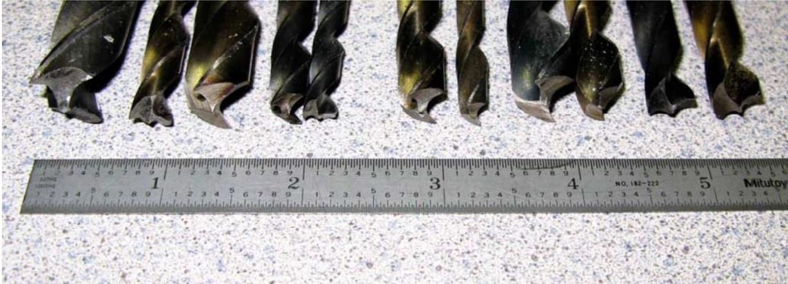
Here are a few of my sheet metal drills. These range from about 3/16" to 5/8" in diameter. If you only drill aluminum, they will stay sharp for quite some time. Use slow speeds on steel, as the tips that cut the diameter have a small cross section and have little mass to dissipate heat. Always use oil when cutting and they will last quite a while before they have to be touched up again, for sharpening. The diagrams and photos will show you how to grind the tip.
