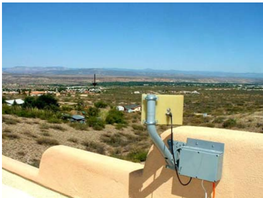
Waterproof box and mounting at far end Arrow showing the other link 1.5 miles away.
